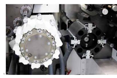
rotates but also makes an oscillating movement. As there are separate servomotors the rotational speed of the can and that of the brush can be set independently of each other. If the machine is equipped with two individual brushing units, each of these units can be controlled separately, a feature that opens up new prospects in the can forming process.
