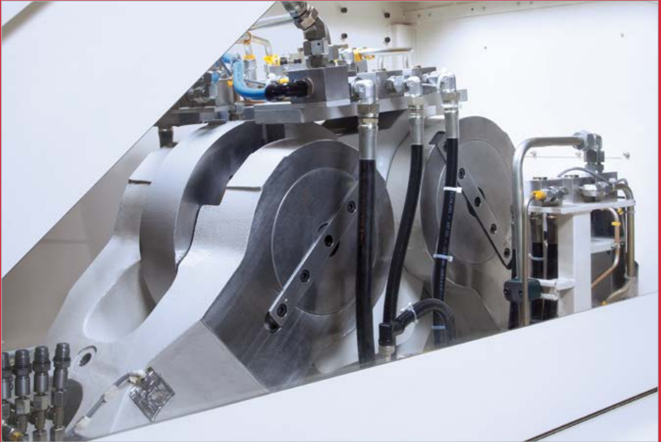
Hinterkopf knuckle-joint drive on an impact extrusion press X-300 S.
