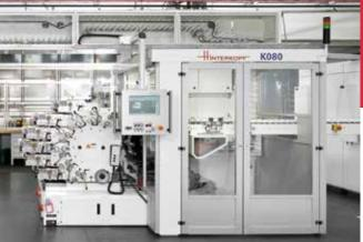
Basic machine for the continuous transfer of the products from and to a transport chain, production speed up to 400 products.
