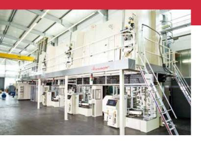
**Thermal drying ovens** or **UV curing systems** are used to fix and harden the applied lacquering or ink layers.
