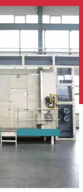
Accumulators represent an important element in the complex production process of tubes and cans. Owing to their capability of buffering products, line parts before and after the accumulator can operate more independently.
