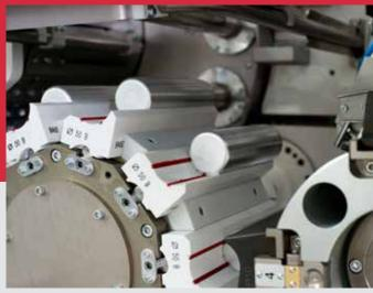
The B240 trimming and brushing machine is based on the H240 basic machine. The 16-station mandrel plate offers plenty of space for the work and monitoring stations, and the wellknown triple transfer from the mandrels onto the continuously running pin chain ensures a smooth running. As in the H240, the transfer unit is driven by a servomotor, its motion can be adjusted to the can length. Short can, short stroke – long can, long stroke.
