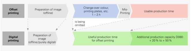
Schematic production process for offset and digital printing
