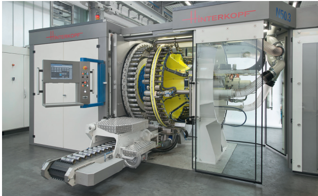
The necking machine N50.3 from Hinterkopf with its 50 working stations opens up entirely new possibilities for shaping.
