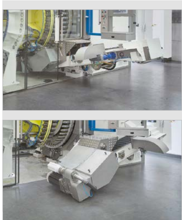
Moveable and adjustable (in height and angle) infeed and exit conveyors for good access.
