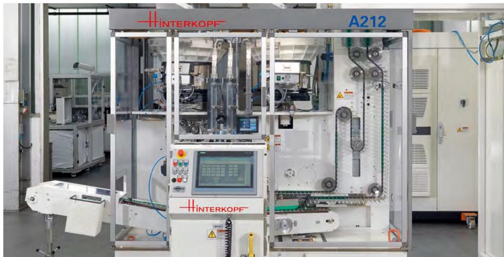
The new A212 is an extremely flexible capping machine for tubes with different caps made of aluminum or plastic.
