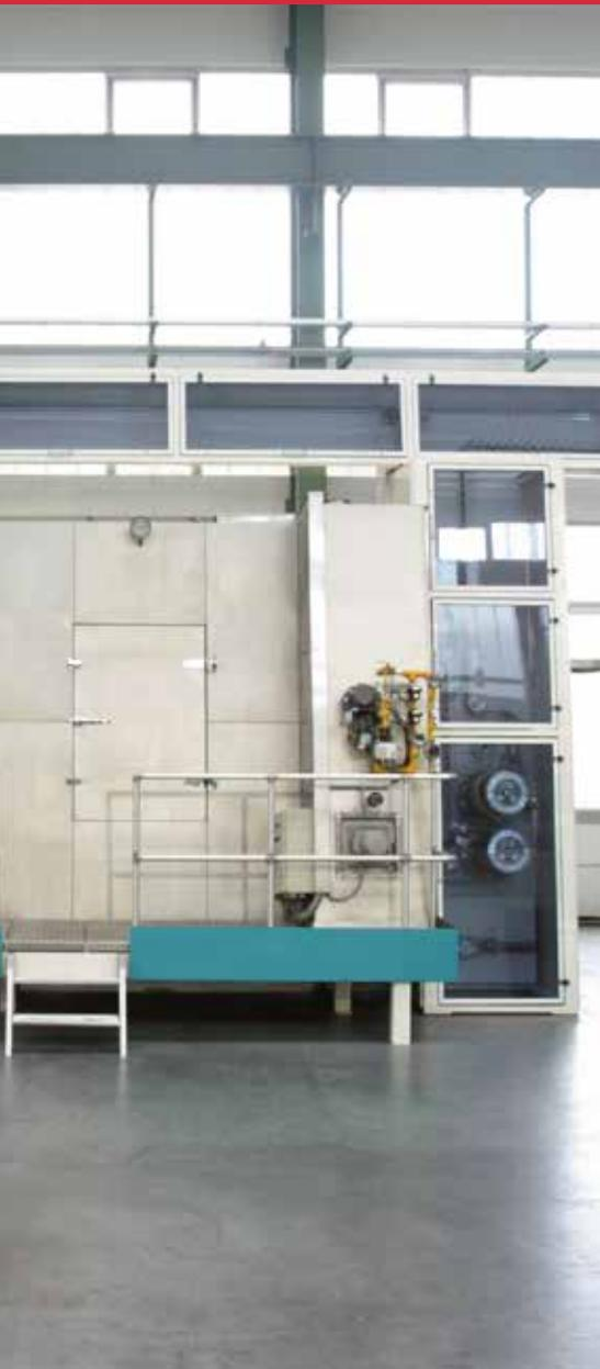
**Accumulators** represent an important element in the complex production process of tubes and cans. Owing to their capability of buffering products, line parts before and after the accumulator can operate more independently.
