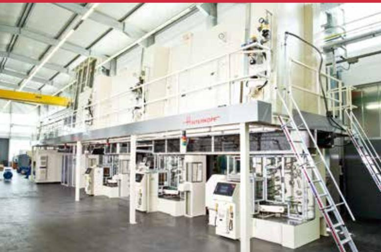
**Thermal drying ovens** or **UV curing systems** are used to fix and harden the applied lacquering or ink layers.
