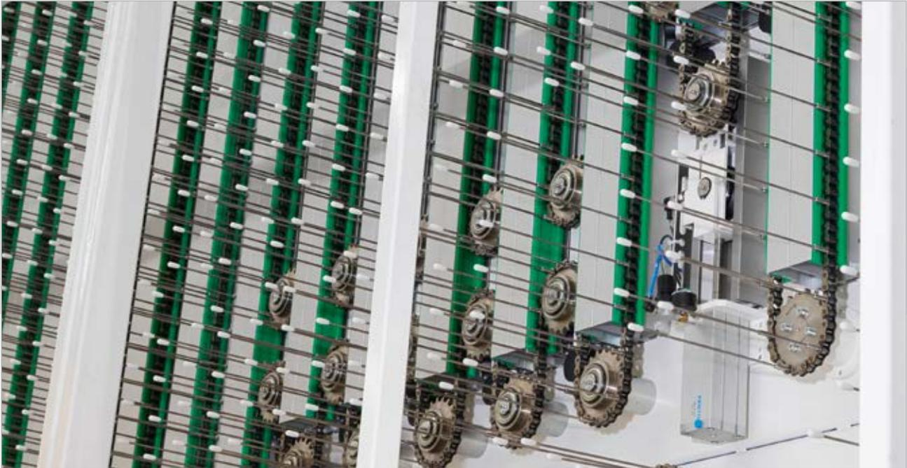
Pneumatic chain tensioners provide for proper chain tension. The chain tension is adjusted by pressure regulators. Proper pressure adjustment is achieved when a smooth chain run is achieved.
