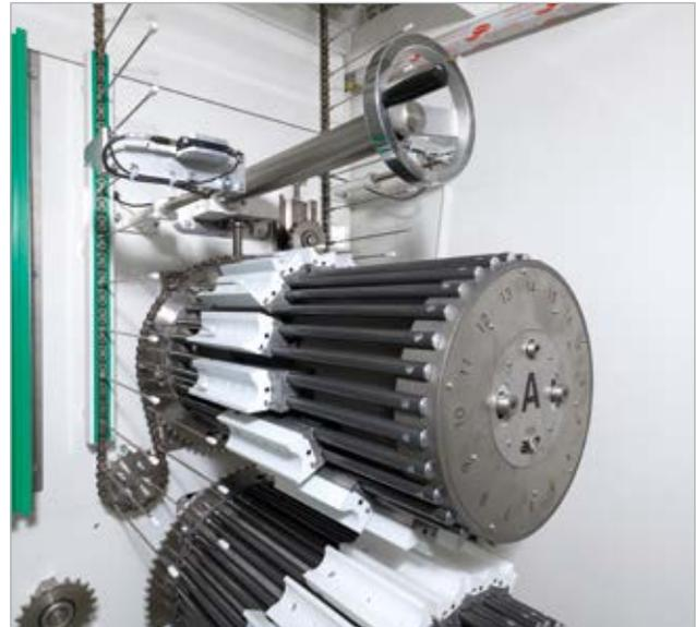
Loading and unloading drums are equipped with vacuum assisted product baskets.
