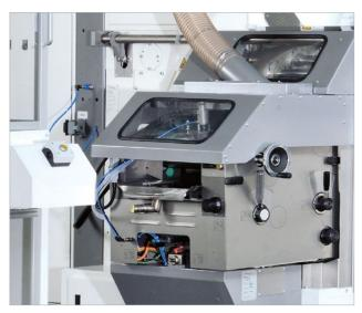
The coating machine receives a stream of inside-sprayed, cured and cooled cans, and applies a base-coat on them in a continuous fashion.
