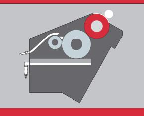
Dipping, rolling or wiping – these are the techniques used on the well-proven lacquering units of HINTERKOPF, installed in its lacquering machines H240L
