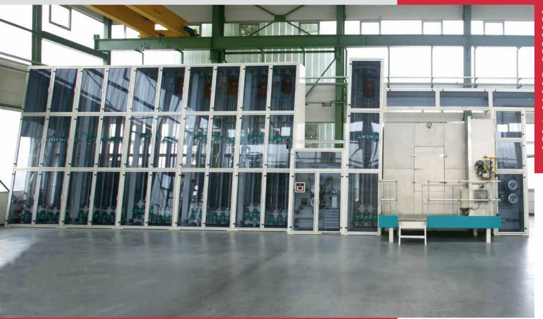
Accumulators represent an important element in the complex production process of tubes and cans. Owing to their capability of buffering products, line parts before and after the accumulator can operate more independently.
