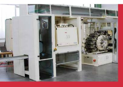
**TS 19** UV curing system in a production line of plastic tubes.
