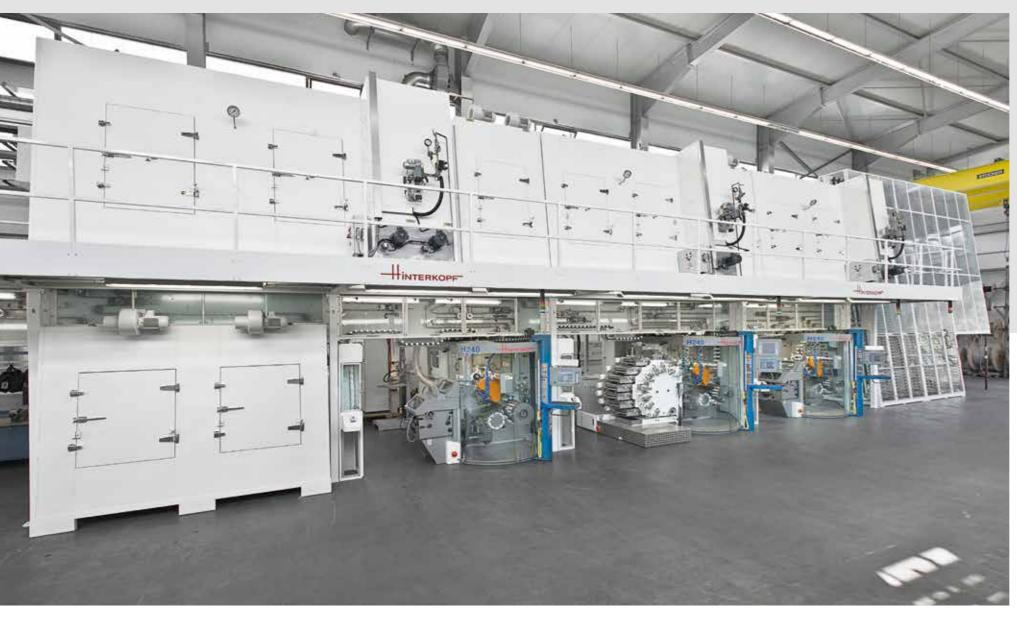
HINTERKOPF offers its customers complete production lines or parts thereof. In a line for aluminum aerosol cans, for example, the fully shaped and decorated can ("Coil-to-Can") is formed from the aluminum blank, the slug.
