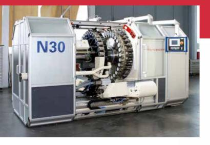
N30 Necking machine for standard cans with 30 work stations.
