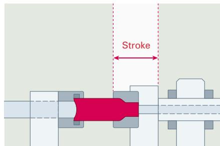
Short stroke for the forming of the upper neck of the can
