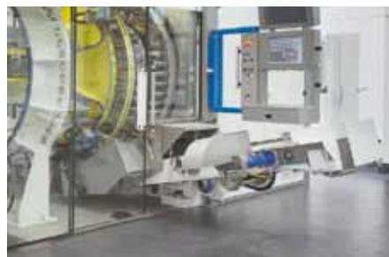
*Moveable and adjustable (in height and angle) infeed and exit conveyors for good access*
