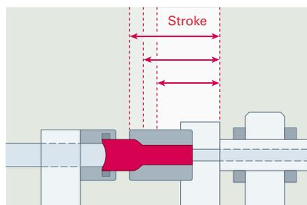
Different lengths of the stroke can be chosen for shaping the can body
